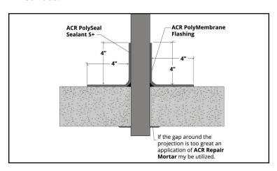
26. Once the sealant has begun to skin over, begin applying ACR PolyMembrane Flashing to all the projections by applying the product with paint roller. Product should be applied at no less than 30 mil dry thickness and should be applied no less than 4" onto the concrete surface and no less than 4" onto the projection. Repeat this process for every projection coming through the surface of the concrete.
