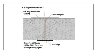
22. Once the sealant has begun to skin over, apply ACR PolyMembrane Flashing over the top of the control joint using a paint roller. Liquid flashing should be applied at least 30 mils dry thickness and at least 4" either side of the control joint.
