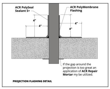
25. Once the sealant has begun to skin over, begin applying ACR PolyMembrane Flashing to all the projections by
